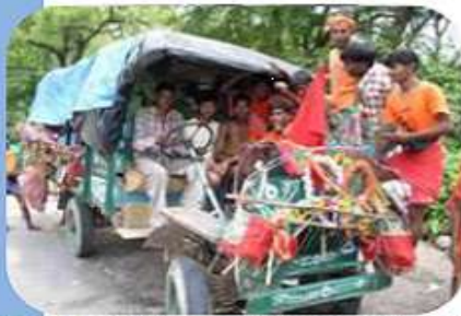
Jugaad, a rural transport vehicle assembled locally with diesel pump as engine and gear assembly of a MUV
